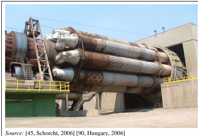
Figure 1.18: Example of a planetary cooler
