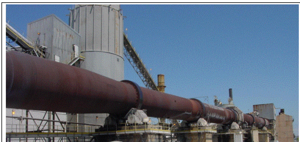
Figure 2.31: Example of a long rotary kiln used in lime manufacture
