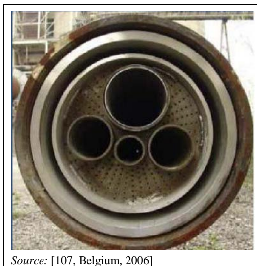
Figure 1.11: Example of a multi-channel burner
