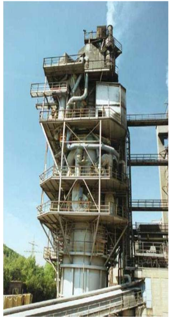
Figure 2.26: Example of an annular shaft kiln used in lime manufacture1 Source: [44, EuLA, 2006]
