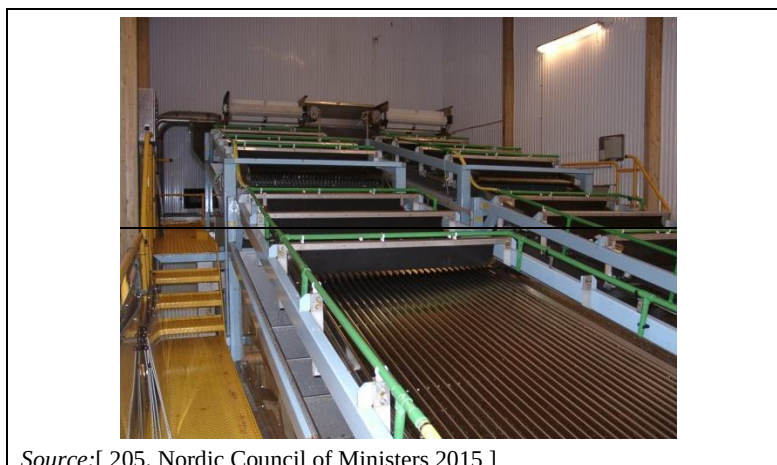
Figure 7.6: Vibrating grading machine
