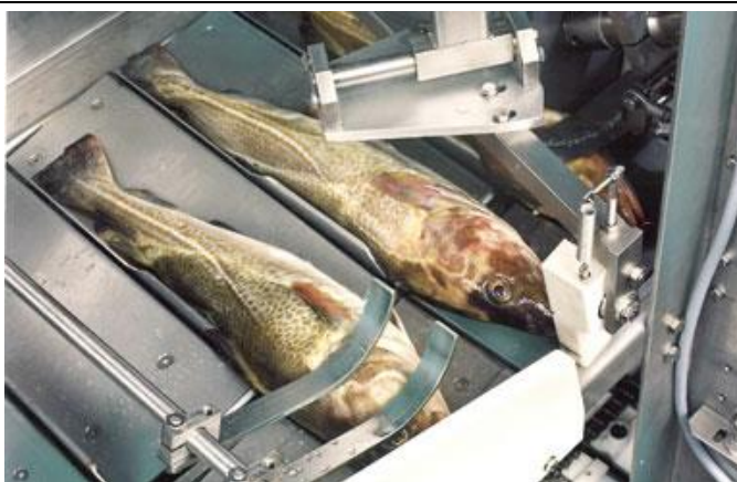
Figure 7.5: Heading, gutting and roe recovery machine
