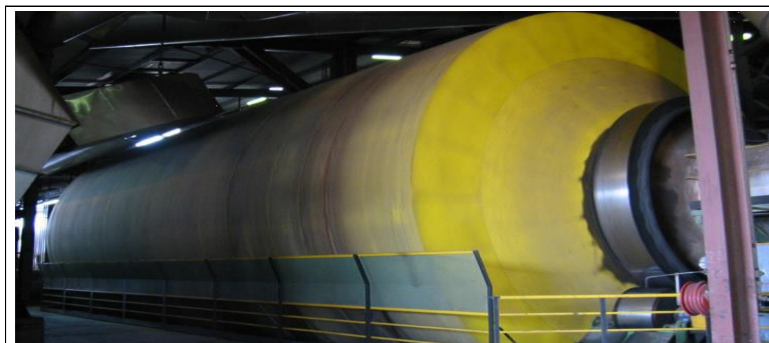
Figure 3.9: Three-pass drying drum
