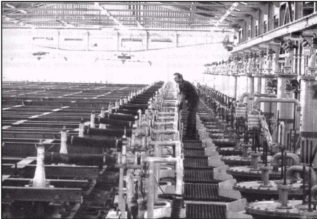
Figure 2.5: Mercury cells with vertical decomposer [Le Chlore, 1996]
